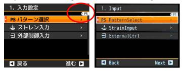
The pattern number being set is displayed as "P5" on the upper right of the setting screen as shown above.
