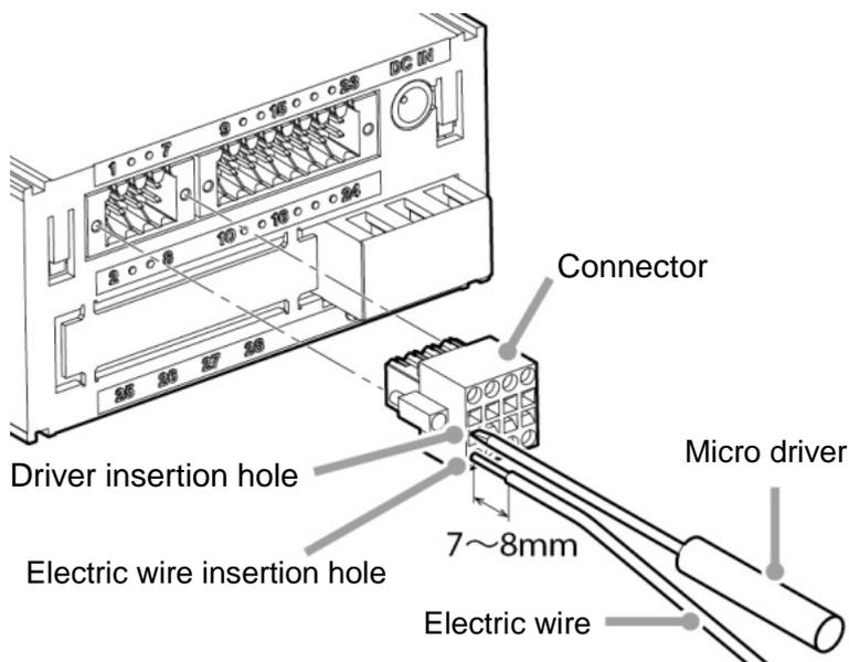
1. Strip wire 7 to 8 mm and twist it enough not to untwist the wire end.
