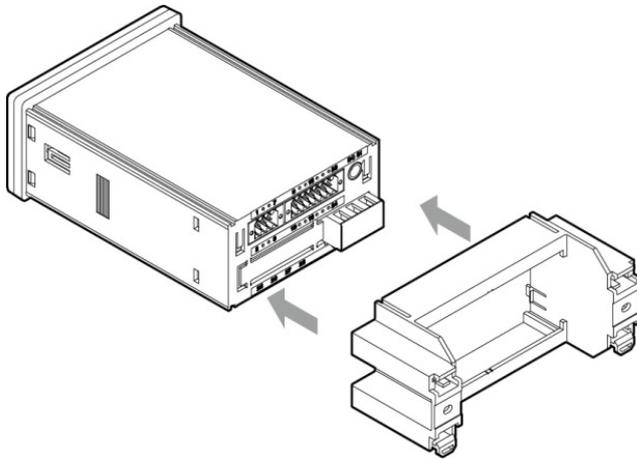
2. Insert the DIN rail adapter diagonally and fix it.
