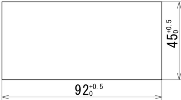
Recommended panel thickness is 0.8 to 5.0 mm.
