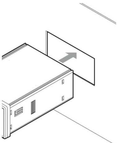
3. Attach left and right panel mounting jigs removed in 1 to the Product rear and fix them.
