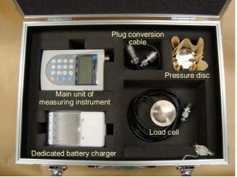
2) Connect the plug conversion cable to the FM-2 measuring instrument.
