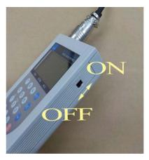
7) Set the display to zero by performing the following operation: Press the 3 key, select 1 (1: SET), and press the (SET/CHG) key. CURRENT DATA ZERO CH1 1 : SET 2 : CLEAR ESC: CANCEL
