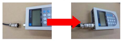
3) Connect the load cell and the plug conversion cable.
